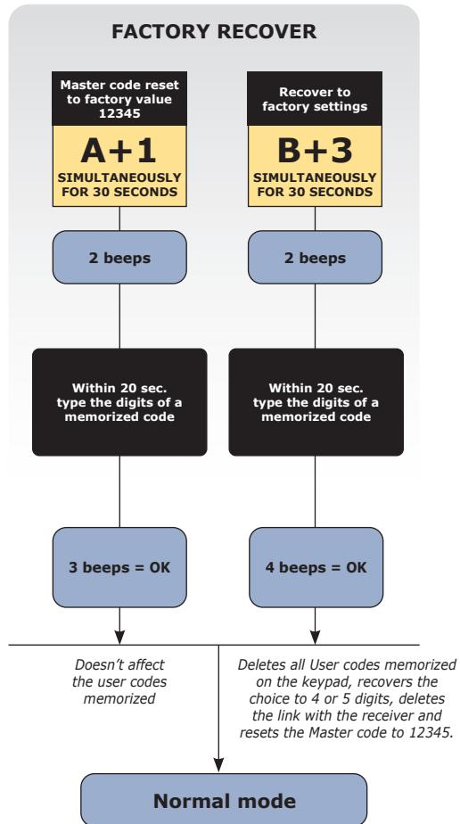
NOTE : At the end of procedure "B+3", even the user code typed within the procedure will be deleted and the keypad must be memorized again onto the corresponding receiver.
