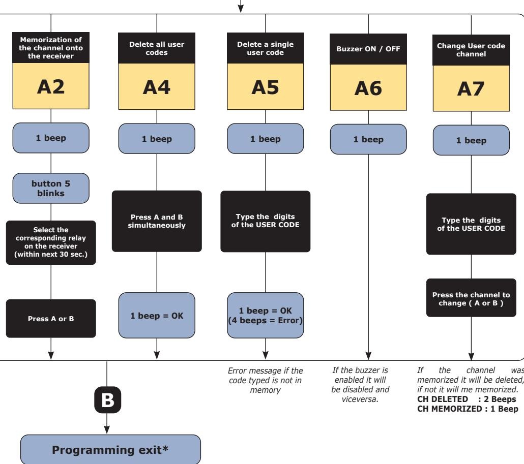
\* The programming mode is limited to 10 sec. without any action on the keypad ( no buttons pressed )
